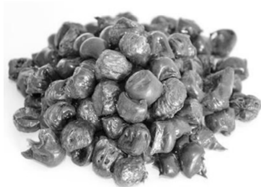
Figure 4. Aggregate produced from PET film Source: author's work.
