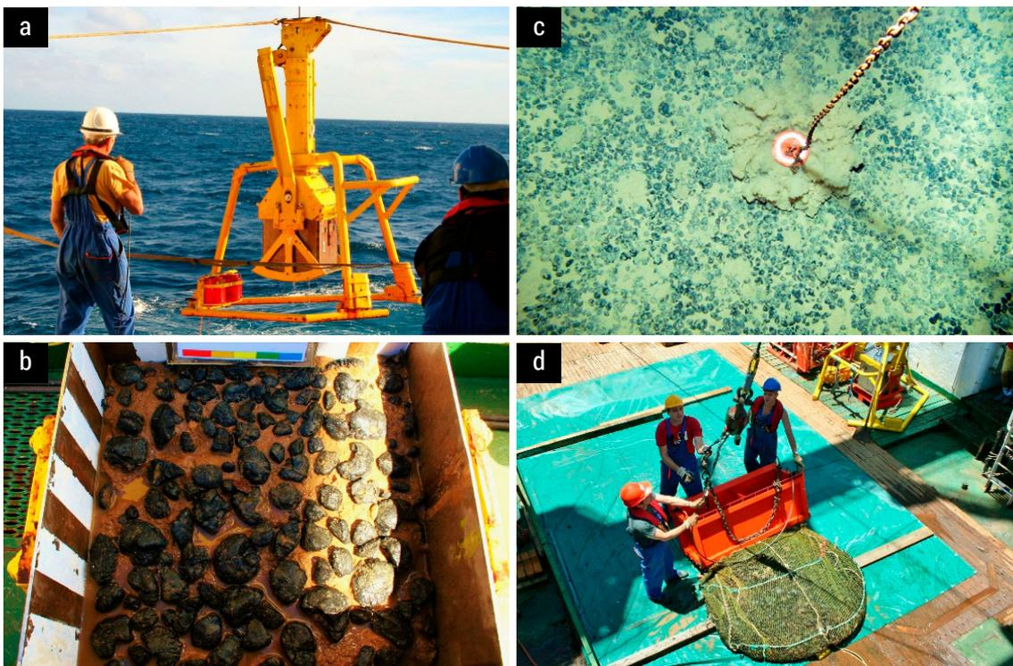
**Figure 3.** IOM exploration activities, a) box corer operations onboard of a research vessel, b) portion of seabed with polymetallic nodules on the surface – view inside a box corer (black and white stripes on the inner sides of box corer are 5 cm wide), c) polymetallic nodules on the seabed – picture from deep sea photo camera (the red-white circle scout on the seabed has a diameter 10 cm), d) collection of approximately 600 kg sample of polymetallic nodules using a trawl
