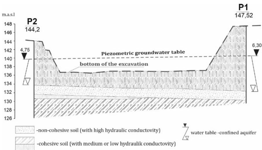
Figure 3. Schematic hydrogeological cross-section through the post-mining excavation – confined aquifer
