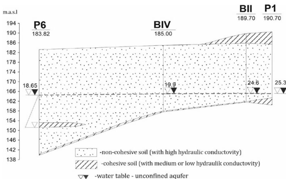
Figure 4. Schematic hydrogeological cross-section – unconfined aquifer
