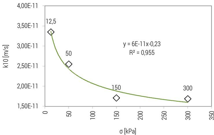
Figure 2. Dependence of the filtration coefficient on the load (varved clay)
