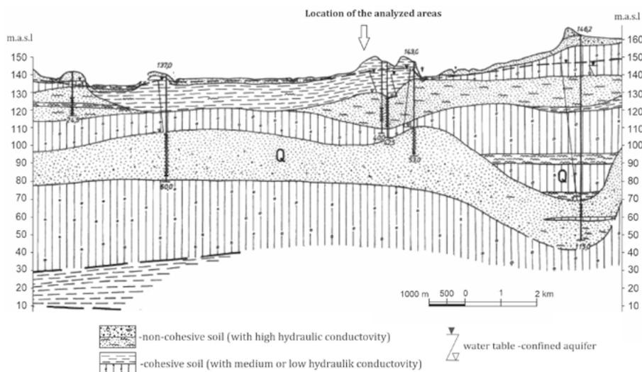
**Figure 1.** Hydrogeological cross-section of the research area
