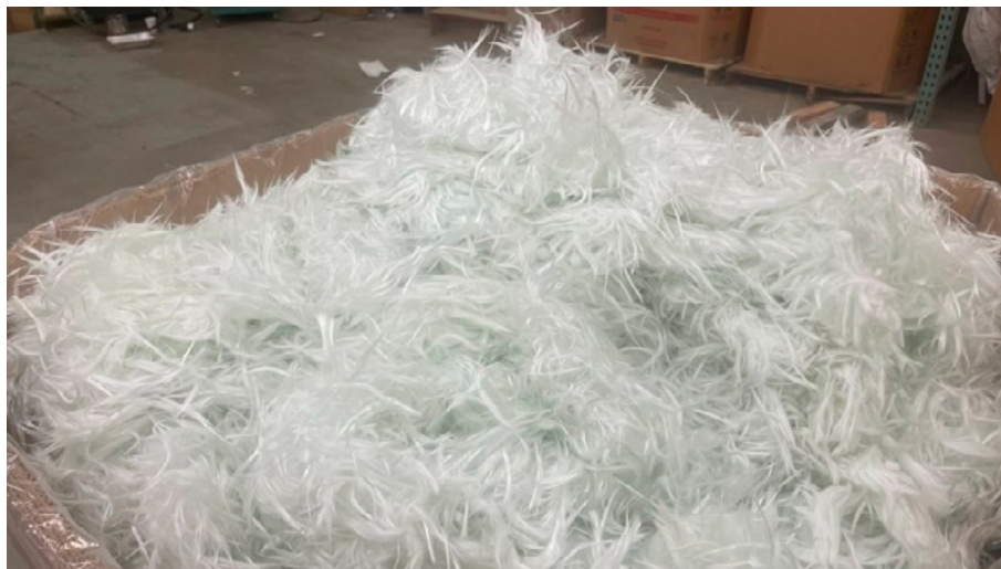
Figure 3. Pure recycled glass fibre from retired wind turbine blades
