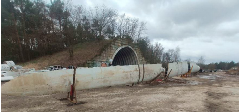
Figure 5. Wind turbine propeller segments with a total length of approximately 30 m Source: Road and Bridge Department, 2020.
