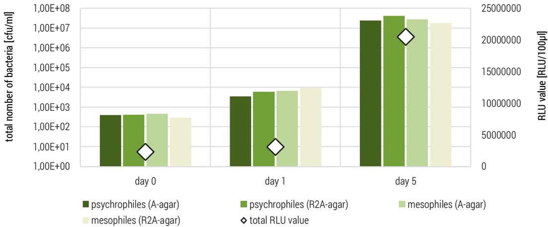
Figure 7. Changes in the total number of bacteria and RLU values in post-fermentation leachate after thermal hygienization at 60°C
