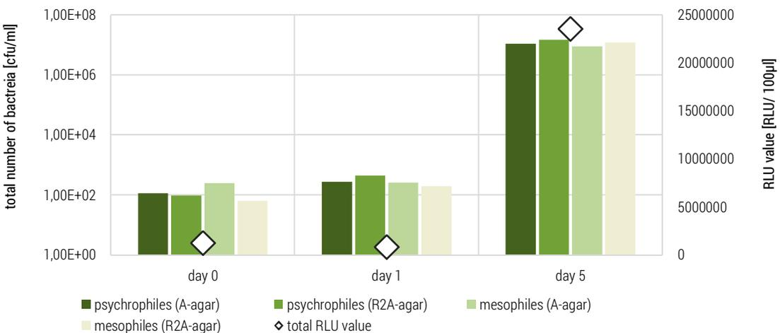
Figure 9. Changes in the total number of bacteria and RLU values in post-fermentation leachate after thermal hygienization at 80°C
