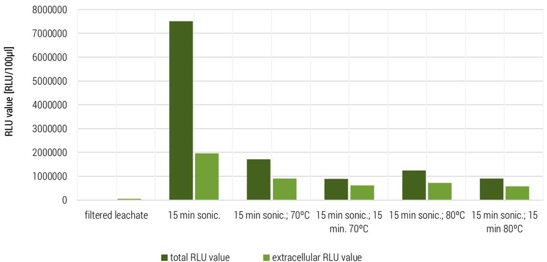
Figure 6. ATP value in the post-fermentation leachate subjected to sonication and temperature
