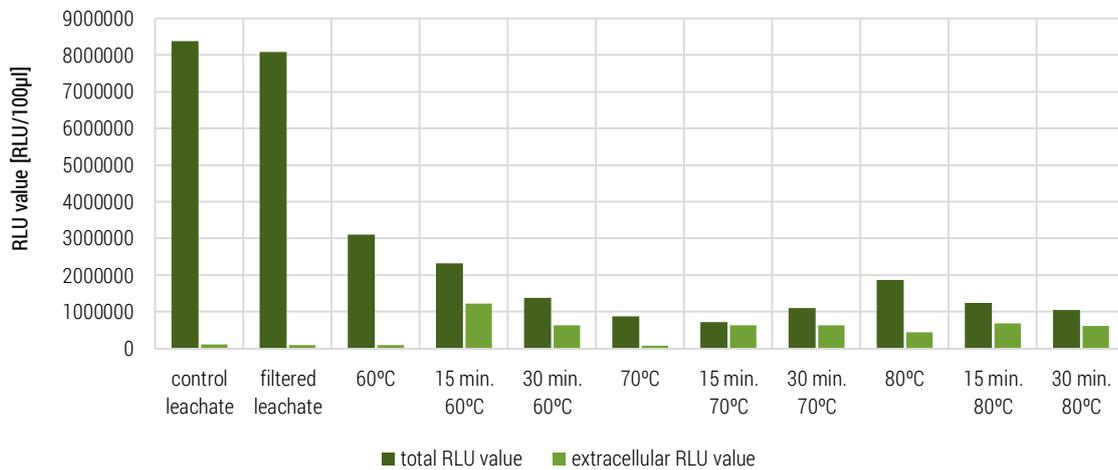
Figure 3. RLU value in post-fermentation leachate subjected to filtration and heating
