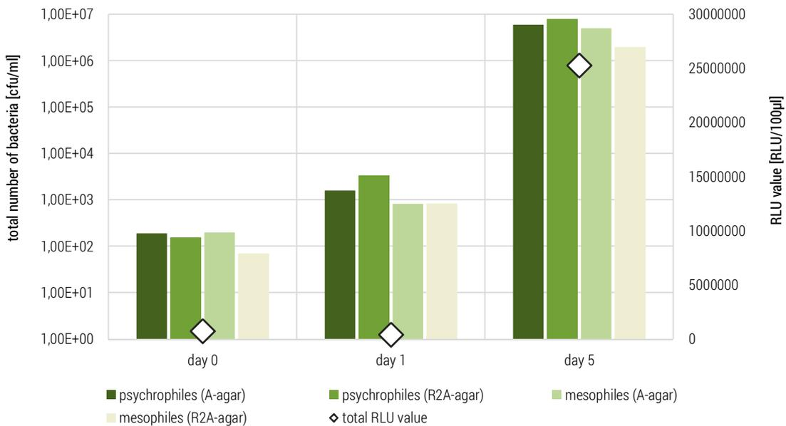
Figure 8. Changes in the total number of bacteria and RLU values in post-fermentation leachate after thermal hygienization at 70°C
