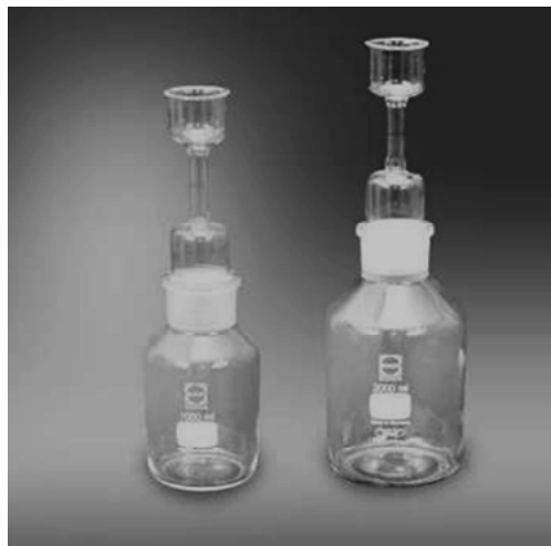
Figure 6. Pycnometer for determining grain density and absorbability
