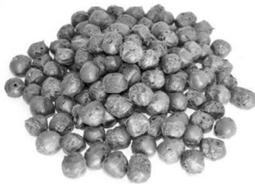
Figure 5. Aggregate produced from a mixture of PET, PVC, and OPS films Source: author's work.
