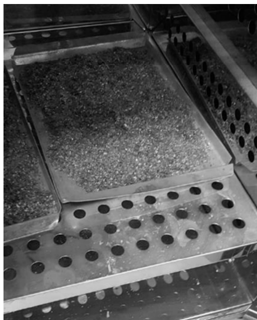
Figure 3. Drying stage of milled plastic to reduce its moisture content
