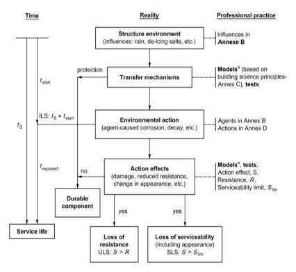
Figure 2. Design durability limit state
