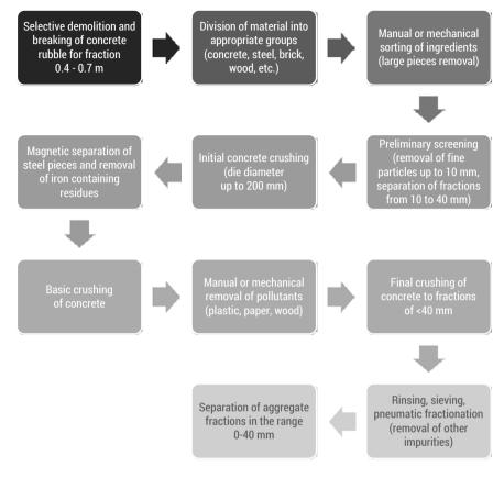
Figure 4. Stages of processing rubble into aggregate
