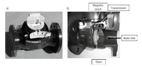
Figure 1. Screw water meter: a) view, b) cross-section Source: author's own work.
