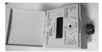
**Figure 3.** Electronic static water meter Source: author's own work.
