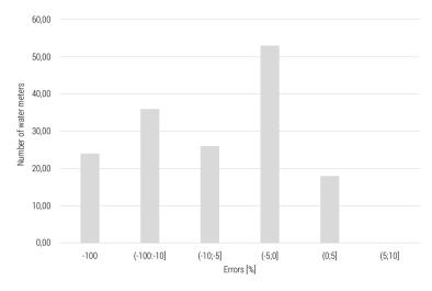
**Figure 4**. Number of water meters in each range of reading errors at the minimum flow rate Source: author's own work.
