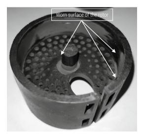
**Figure 10.** Worn side of the piston in a volumetric water meter Source: author's own work.
