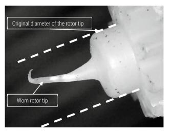
**Figure 9**. Worn rotor axis of a water meter working at a hydrant base Source: author's own work.
