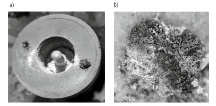
Figure 6. Magnetic coupling of a screw water meter a) view of a magnetic coupling surface with precipitates, b) a microscopic view
