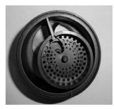
**Figure 2.** Rotor of a volumetric flow meter Source: author's own work.
