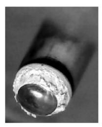
**Figure 8.** Tip of the rotor axis of the single-jet water meter with a diameter of 20 mm Source: author's own work.
