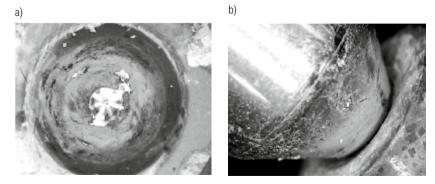
**Figure 7.** Bearing of the rotor of an industrial single-jet water meter covered with scaling a) microscopic view of a bearing with scaling, b)microscopic view of a bearing profile Source: author's own work.
